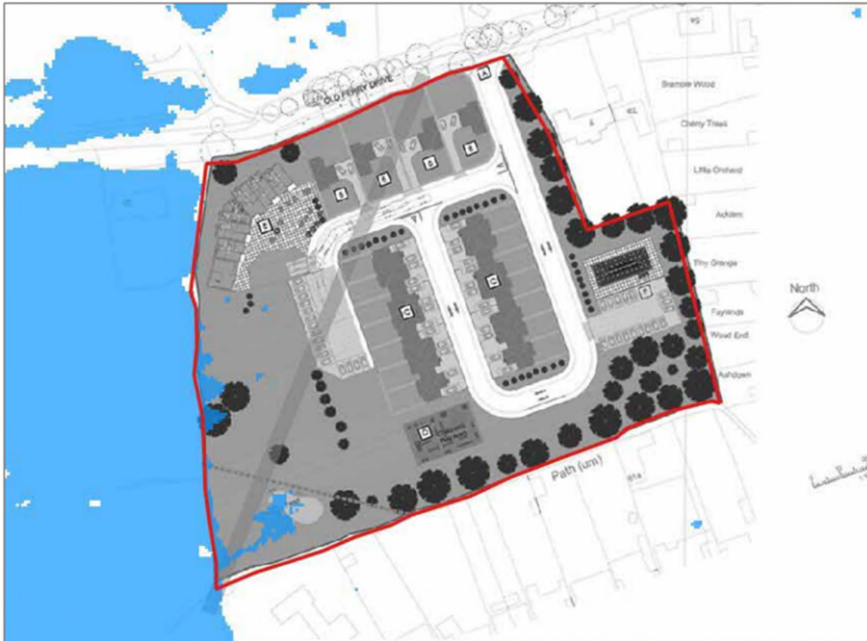
Figure 1 – Extent of flooding during a 1 in 20 year return period event, plotted using 1m resolution aerial height data ((© Environment Agency, Contains Ordnance Survey data © Crown copyright and database right 2021)).
